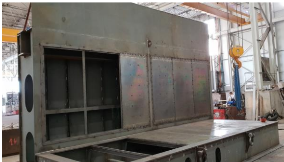
Figure 1. Prototype – Load section of an inland container vessel made with aluminium foam-sandwiches.
