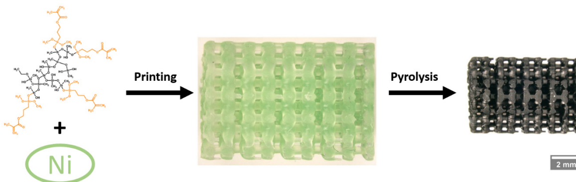
Figure 1. Manufacturing of metal-modified, polymer derived ceramic lattice structures via stereolithography
