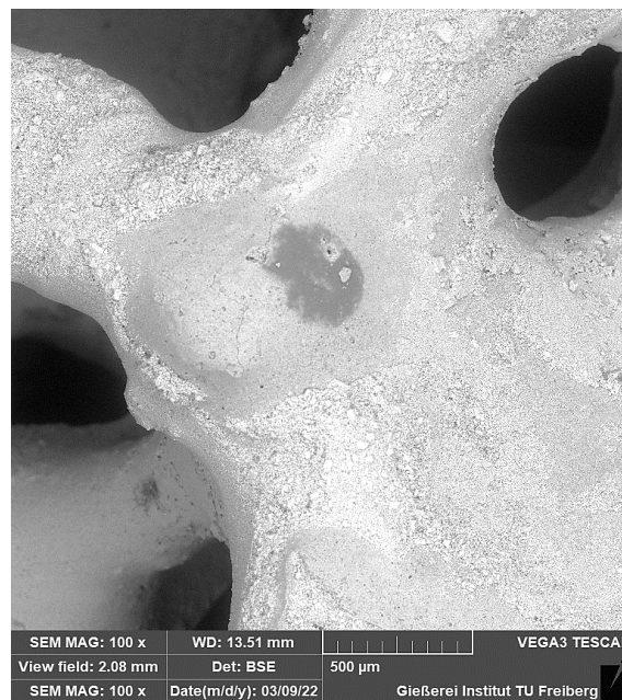
Figure 1: SEM image in backscattered electron contrast (BSE) of the surface of a C-bonded \text{Al}_2\text{O}_3 CFF with MgAlON coating at a magnification (MAG) of 100 times and a working distance (WD) of 2.08 mm.
