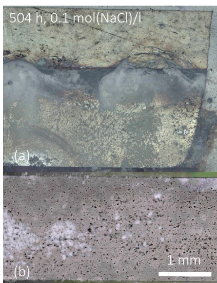
Fig. 2: Corrosion products after corrosion exposure test (a) CFRP-Al hybrid system and (b) Al.
