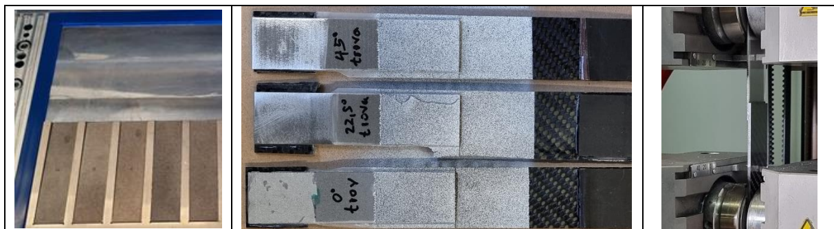
Figure 1. Left: Adapted VARTM mould, Middle: Tensile-shear specimens, Right: Tensile-shear testing.
