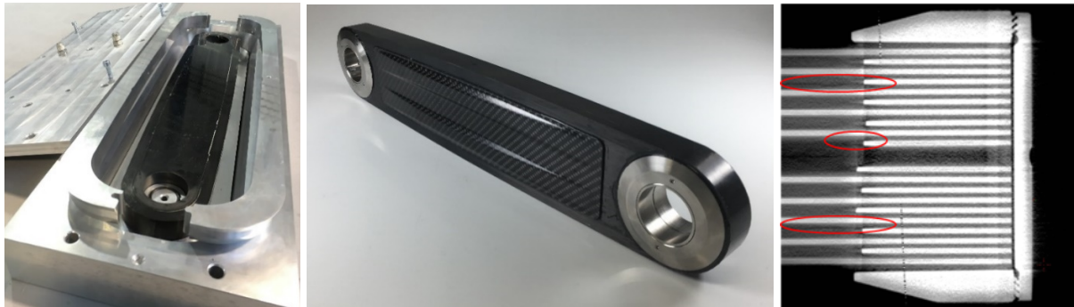
Figure 2. left: infiltrated CFRP-Ti structure in the RTM mold, middle: final scaled drag brace, right: CT picture of a tested specimen (modified after [1])
