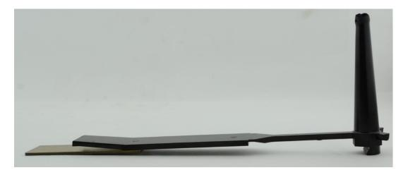
**Figure 1.** Test specimen based on DIN EN 1465 "Adhesives - Determination of tensile lap-shear strength of bonded assemblies"
