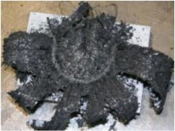
Abbildung 1 Test setup, execution and crushed CFRP omega specimen after the quasi-static compression test, from [3].
