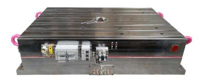
Figure 1. Hot runner intermediate plate  $2,000 \times 1,400 \times 240$  mm with spacer plate  $2,200 \times 1,400 \times 270$  mm. Heat insulation plate (red) between hotrunner and spacer plate.
