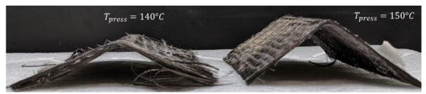
Figure 2. Comparison of preform stability after different preform temperatures with K140 blends.
