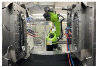
Figure 1. Continuous fiber-reinforced loop as insert in injection mold with force introduction sleeves
