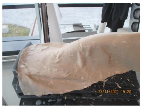
Fig. 1: Initial draping trial, with flakes of the matrix falling of the fibre reinforcement (bottom right)
