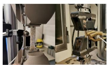
Figure 1. Test-setup for fatigue testing of 3D-printed endless-flax fibre reinforced polylactide at different strand/fibre orientations and R-values (R): (a) UD0, R=0.1 and (b) UD90, R=-1.
