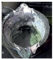
Figure 1. Used casting crucible with ceramic fabric lining (Source: Metallgießerei Chemnitz).
