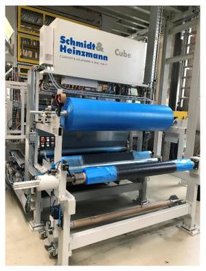
Figure 2. SMC line at Fraunhofer ICT [nonwoven feed (left); SMC semi-finished product (right)] (Source: Fraunhofer ICT)
