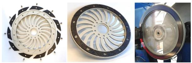
Figure 1: Metal-ceramic hybrid brake disc prototype (outer diameter = 410 mm): Individual parts (left), assembly (middle), prototype during tribological testing (right). [1]
