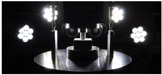
Figure 1. Compression test rig and 3D camera system for mechanical characterization of investigated layer systems.
