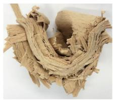
**Abbildung 2.** Test set-up, execution and crushed omega specimen from layered wood veneer laminate after the quasi-static compression test.
